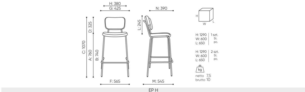
**B** seat height: measured according to the norm
