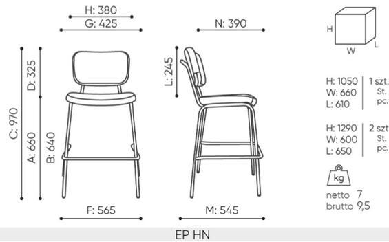
**B** seat height: measured according to the norm PN EN 1335-1 with a load of 640N
