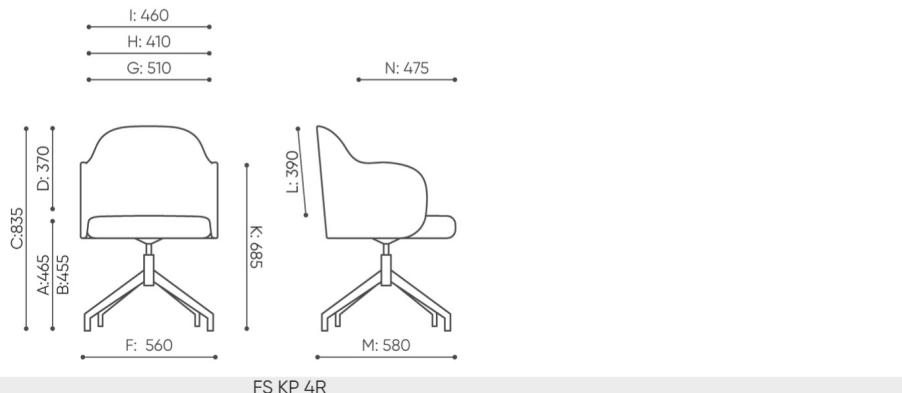
**B** seat height: measured according to the norm
