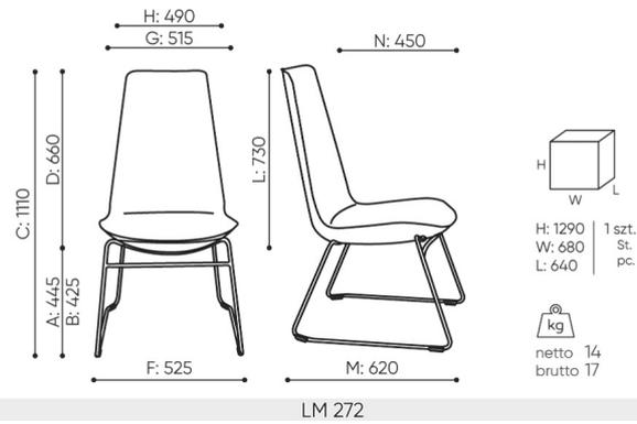
**B** seat height: measured according to the norm PN EN 1335-1 with a load of 640N
