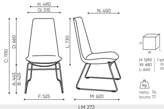
**B** seat height: measured according to the norm
