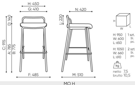
**B** seat height: measured according to the norm
