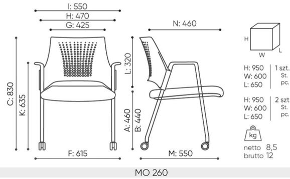
**B** seat height: measured according to the norm PN EN 1335-1 with a load of 640N
