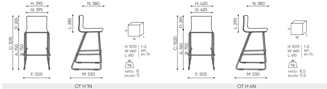
**B** seat height: measured according to the norm PN EN 1335-1 with a load of 640N
