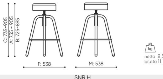
**B** seat height: measured according to the norm
