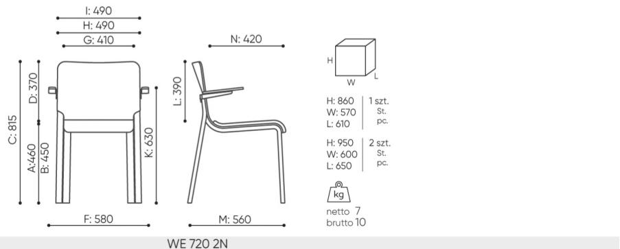
**B** seat height: measured according to the norm
